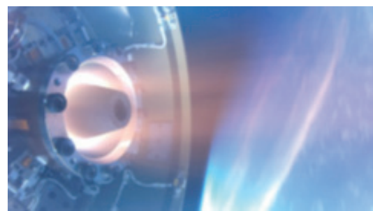
In-space Rotating Detonation Engine demonstration (courtesy Nagoya University)
