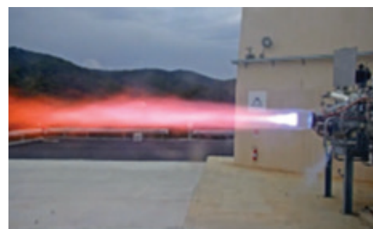
Firing test of the M10 engine (courtesy AVIO S.p.A.)
